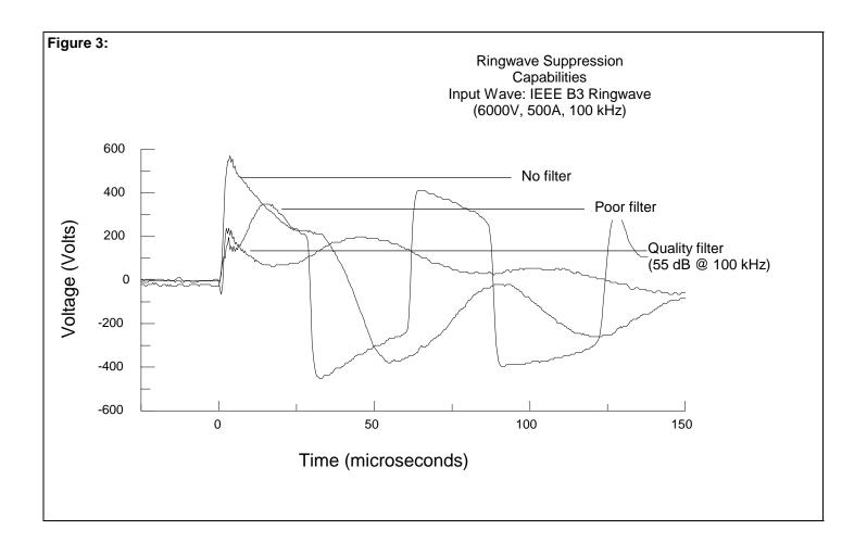
In addition, a system wide suppression design provides enhanced normal mode and common mode noise attenuation - significantly greater than a stand alone device. representative or our Customer Service personnel (1-403 277 2255) for any questions concerning technical suppression or application assistance.
